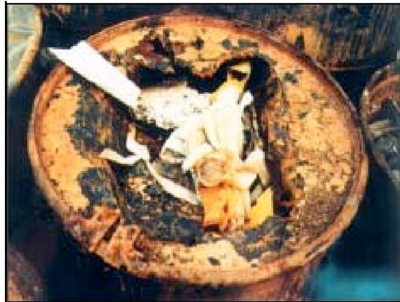
*Damaged and leaking waste barrels inside CSM*
